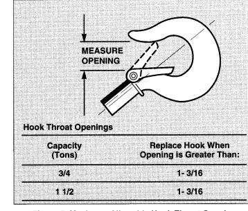
Figure 5. Maximum Allowable Hook Throat Opening
