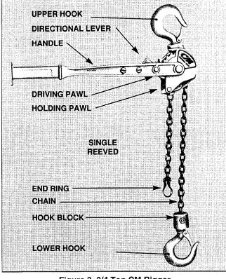
Figure 3. 3/4 Ton CM Rigger
