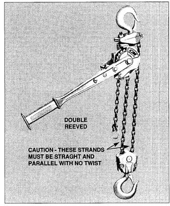
Figure 4. 1 1/2 Ton CM Rigger
