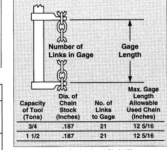
Figure 6. Gaging Load Chain Wear
